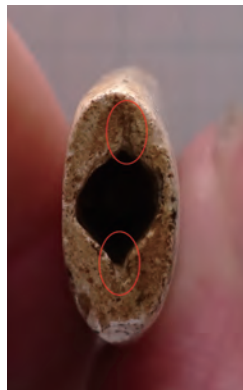
Fig.23 End cut with grooves
