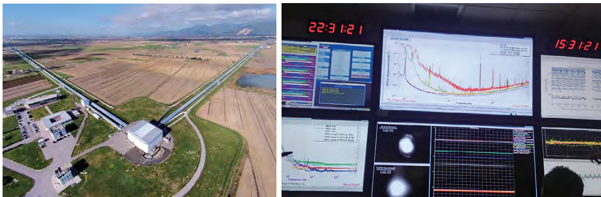
Figure 28. Laser Interferometer Gravitational-Wave Observatory (LIGO), the left plot showing two 4-km long vacuum tubes for gravitational wave measurements, and the right plot showing data of the first gravitational wave detected by LIGO
